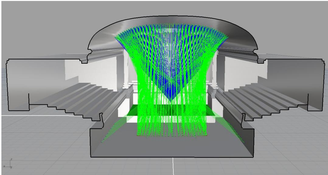
**Figure 2: 3D raytrace of the concave ceiling of Kulturcasino, Bern (cross-section view), showing that a large portion of the parterre width is covered by mild focusing from the ceiling.**
