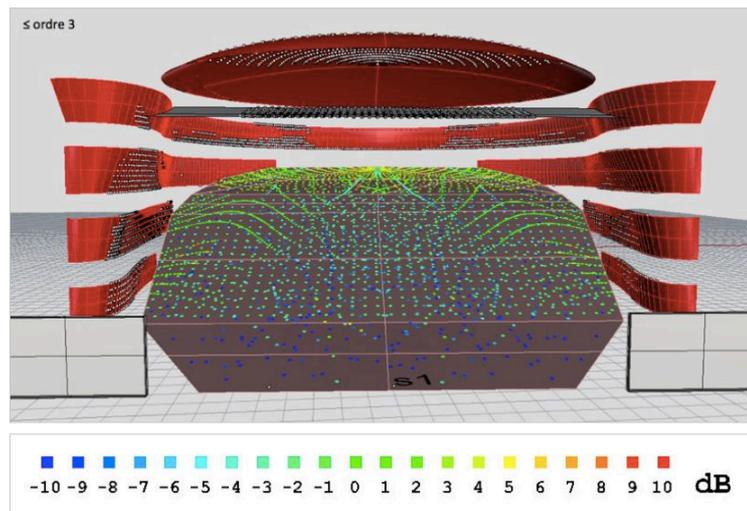
**Figure 5:** combined focusing study of the proposed bands and dome of the Comédie, showing the reflection coverage for reflections up to 3<sup>rd</sup> order, for a source 3m behind the stage edge.
