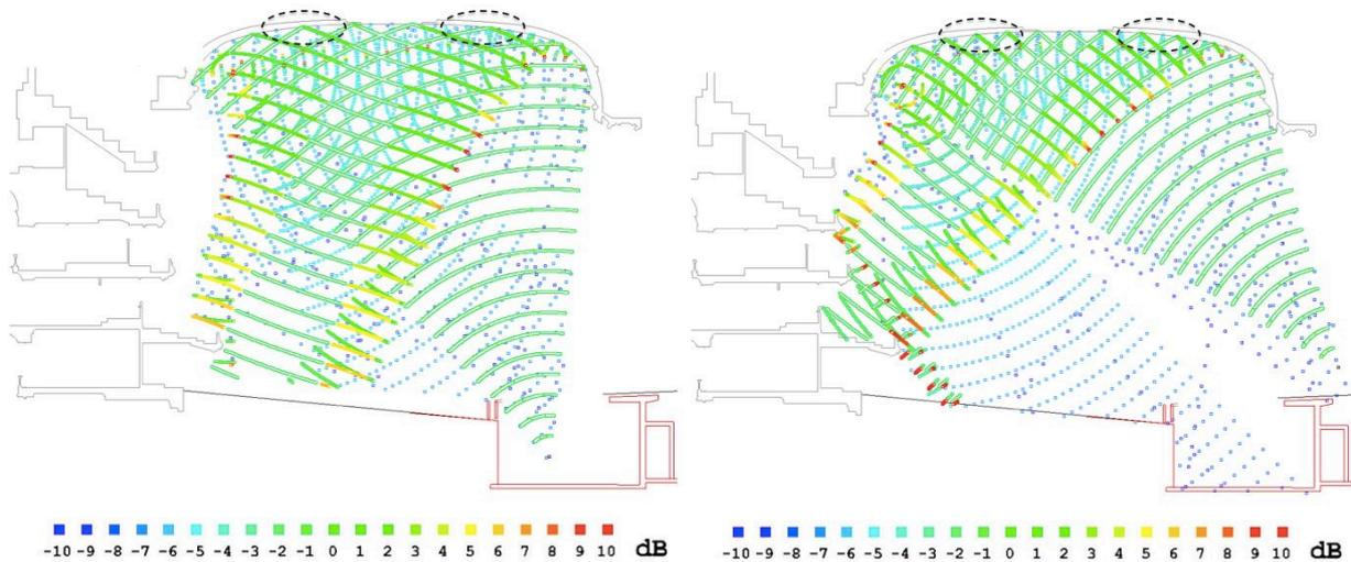
**Figure 1: Long-section showing the focusing effect of the dome of La Monnaie opera house, for a source in the orchestra pit (left image) and on stage (right image). The parameter plotted is  $\Delta L_{\text{curv}}$ . The parts of the dome creating the strongest focusing in the audience are indicated by dashed ovals.**
